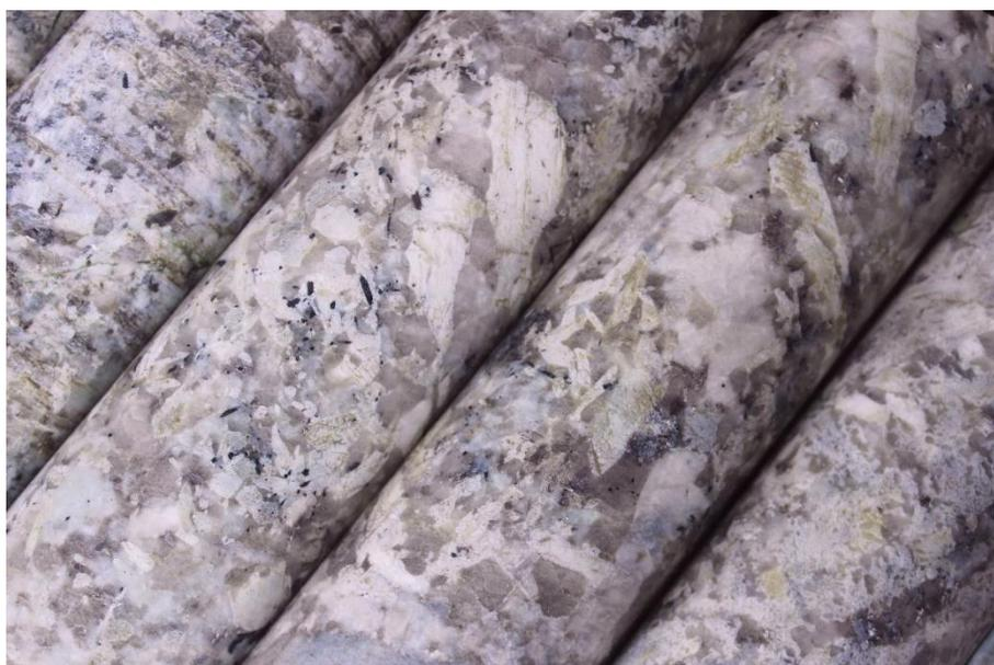
Figure 1: Coarse grained spodumene within KEGM004
